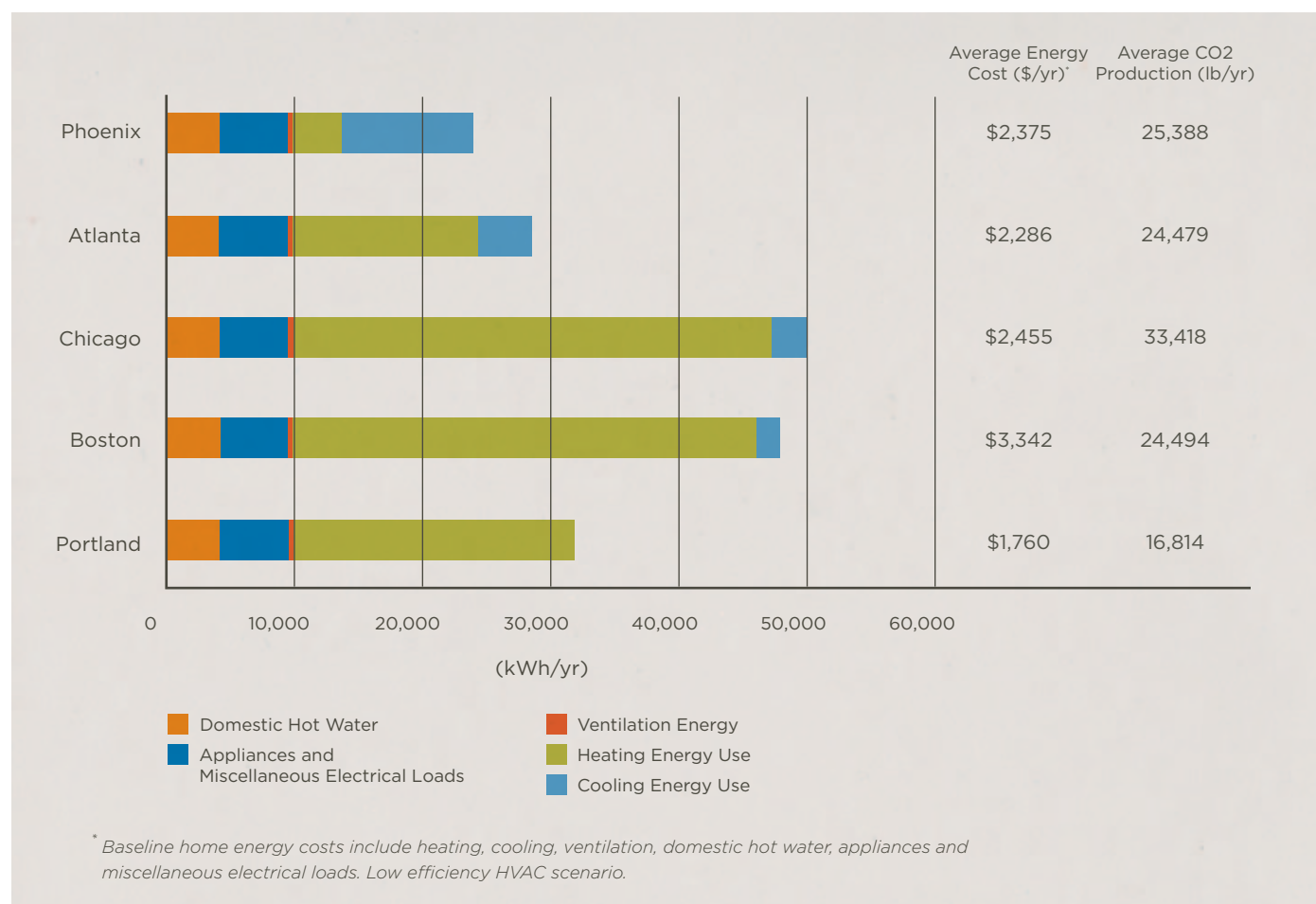
Figure 6: Baseline Annual Energy Use, Energy Cost and CO2 Emissions for the Prototype Home by City
