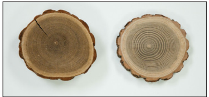
These two tree stems are roughly the same diameter but the slower-grown sample (left) will have a lower proportion of juvenile wood.
