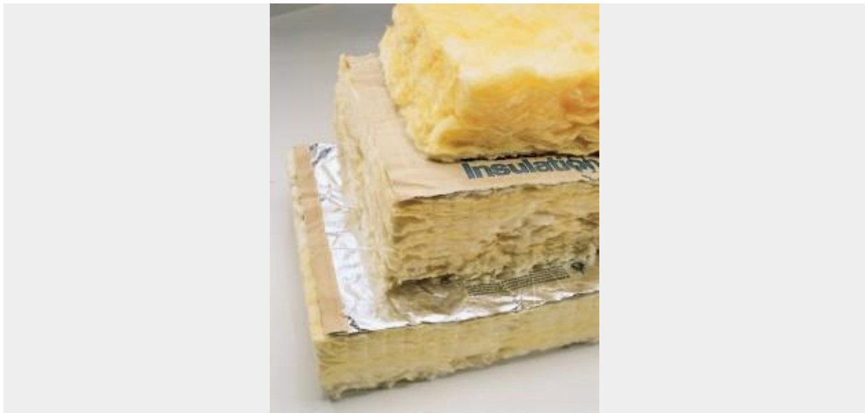
Fiberglass insulation is often faced with kraft paper (the same material used for paper grocery bags); in some products, the kraft paper comes asphalt-impregnated and coated with foil, a facing that is intended to block the movement of moisture. (Photo: Rob Huntley/Lightstream)
